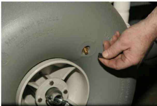
PHOTO 3: REMOVING TIRE VALVE CAP
